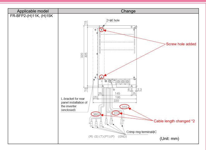
\*2 Check the following tables for the cable lengths before and after the change.
